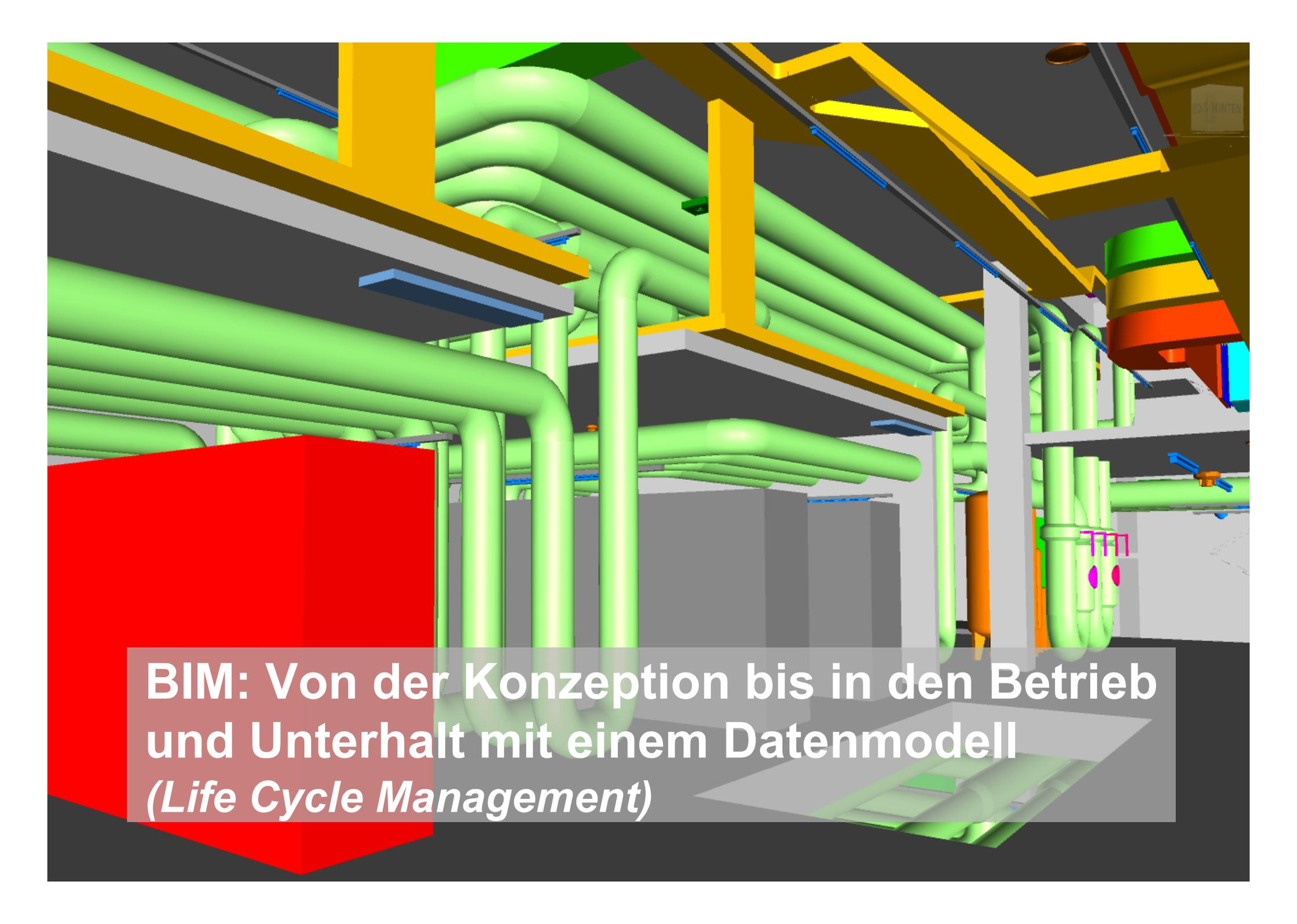
A 3D BIM model of a building's mechanical, electrical, and plumbing (MEP) system. The model features a complex network of green pipes and ducts, yellow structural beams, and grey concrete elements. A prominent red rectangular block is visible in the lower-left foreground. The scene is set within a virtual building environment with a dark floor and ceiling.
